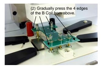
Fig. 4-10 Attaching a B coil
