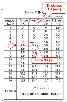
Fig. 4-14 Slider Position No. Table
