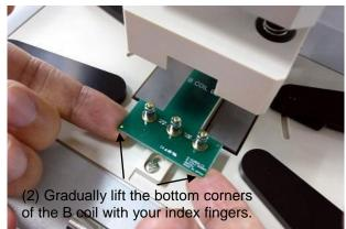
Fig. 4-12 Detaching a B coil
