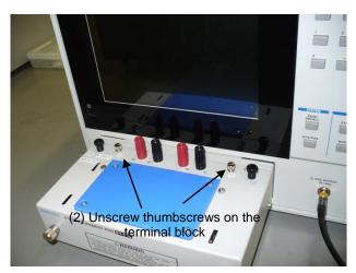
Fig. 4-3 Removing the measuring terminal block
