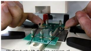
(2) Gradually lift the top corners of the B coil with your index fingers.
