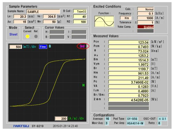
Fig. 4-20 3rd Measurement Screen
