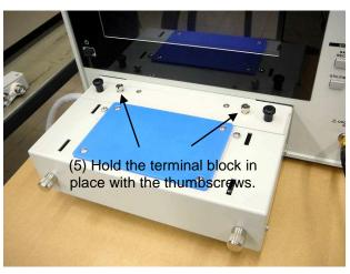
Fig. 4-7 Securing the SY-957 terminal block
