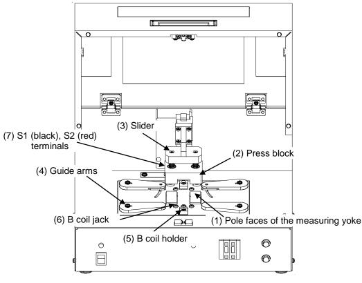
Fig. 3-2 Fixture of the SY-956
