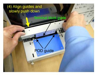
Fig. 4-6 Inserting the SY-957 terminal block
