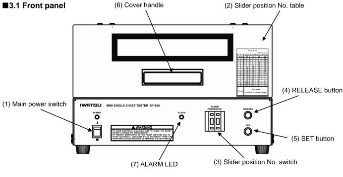
Fig. 3-1 Front Panel of SY-956
