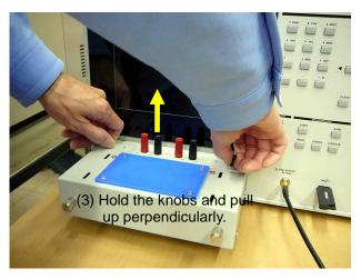
Fig. 4-4 Removing the measuring terminal block
