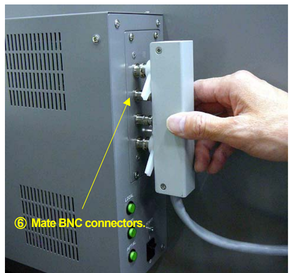
Fig.2-8 Connection of chamber cable
