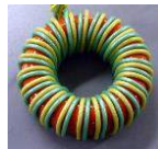
Fe-Based amorphous core L=311 \mu H
