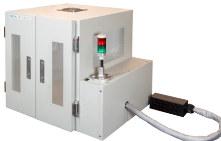
Test Fixture L CS-305 Cooling fan, LED light, Warning light, Power supply outlet and Interlock are equipped. External dimensions: 630Wx520Hx530D(mm)
